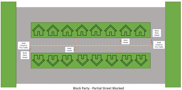
For block parties not closing the entire block, intersection to intersection, barricades and appropriate signage will be delivered by the City. The six barricades and signs should be setup as illustrated, notifying drivers about road closure ahead.
