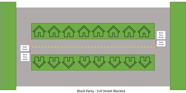
Block Party - Full Street Blocked For block parties closing the entire block, intersection to intersection, barricades and appropriate signage will be delivered by the City. Barricades and signs should be setup as illustrated, notifying drivers about road closure ahead.
