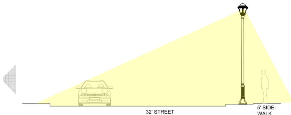
Image 11: Collector/Medium Streetlighting Profile
